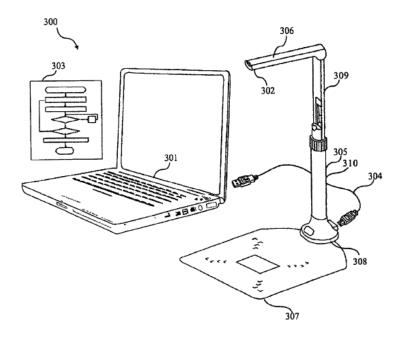
Figure 3a illustrates a document imaging system including personal computer 301 programmed with software 303, and miniaturized video camera 302 mounted so that it can capture images documents placed on surface 307. *Id.* at col. 4, 1. 66–col. 5, 1. 34. Not shown, but referred to as exemplary output displays, are projector and monitor displays. *See id.* at col. 3, 11. 30–34.
