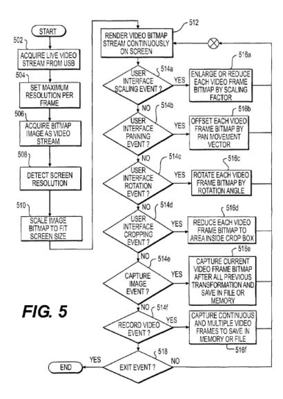
Figure 5 illustrates the acquisition at the computer of a live video stream from the camera via a USB connection, the acquisition of the video stream as a bitmap image, the scaling of the bitmap image to fit the output screen resolution, the rendering of the scaled image on the display, the various image manipulation events performed on the image in real time, including
