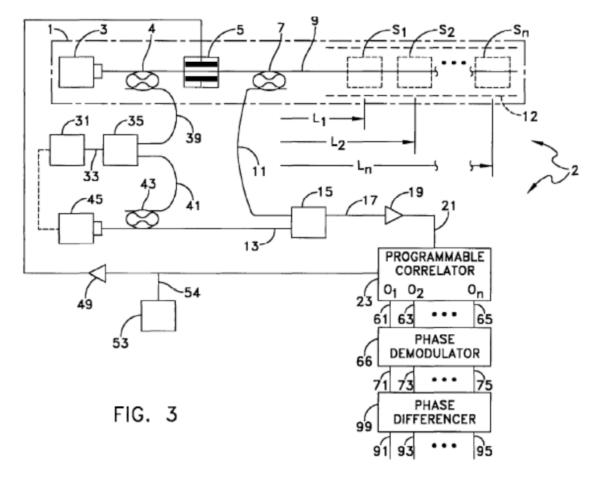
Figure 3 of the '884 patent shows a block diagram of a time-domain reflectometer system.
