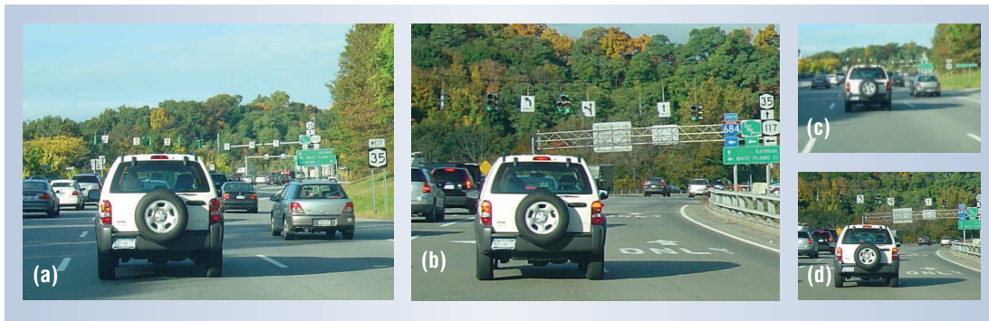
Figure 7. Trip navigation using preloaded images. This system downloads archived images that show (a) the view before a designated turn and (b) the view closer to the turn, showing the driver exactly when to make a required turn. (c and d) Unfortunately, the small size of the integrated camera display view reveals the need for larger displays.
