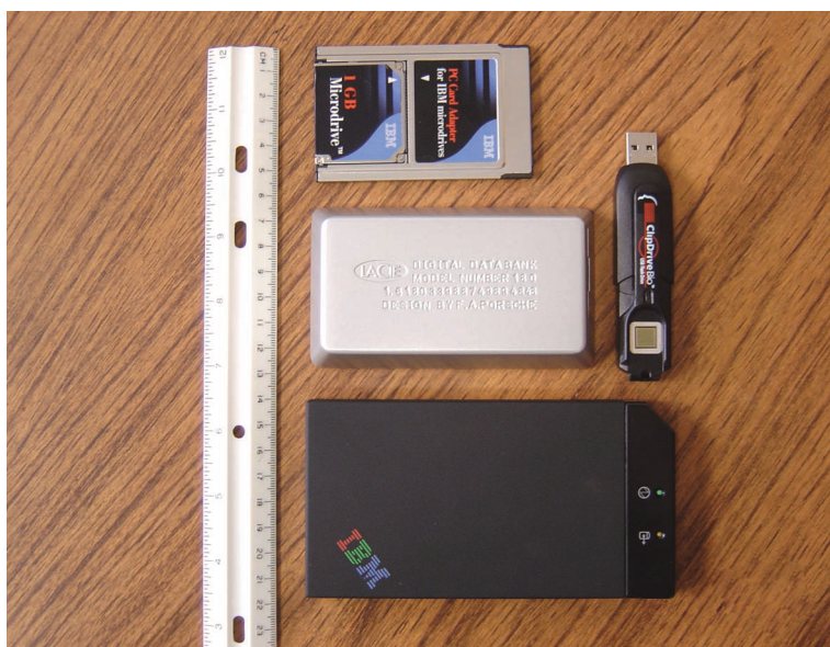
Figure 2. Portable-storage devices with capacities ranging from 512 Mbytes to 40 Gbytes.
