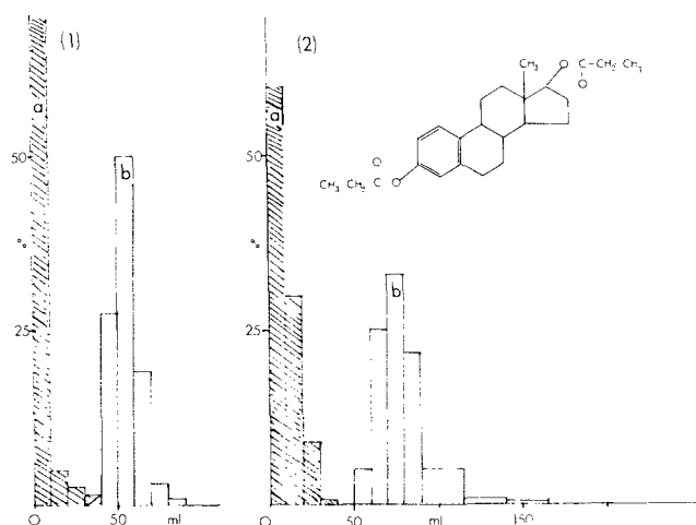
FIG. 7. Separation of estradiol dipropionate from sesame oil. Column 25 x 300 mm. (1) 8.0 g Celite 545 A.W., 9.0 ml nitromethane; (2) 15.0 g Celite 545 A.W., 17.0 ml nitromethane-90% methanol 1:1, mobile phase n -heptane. (a) Sterol and glyceride fractions; (b) estradiol dipropionate.
