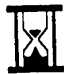
Figure 49. Hourglass Pointer. The mouse pointer changes shape to an hourglass pointer to graphically show users that a user-requested computer function is in process and that additional user requests cannot be accepted.
