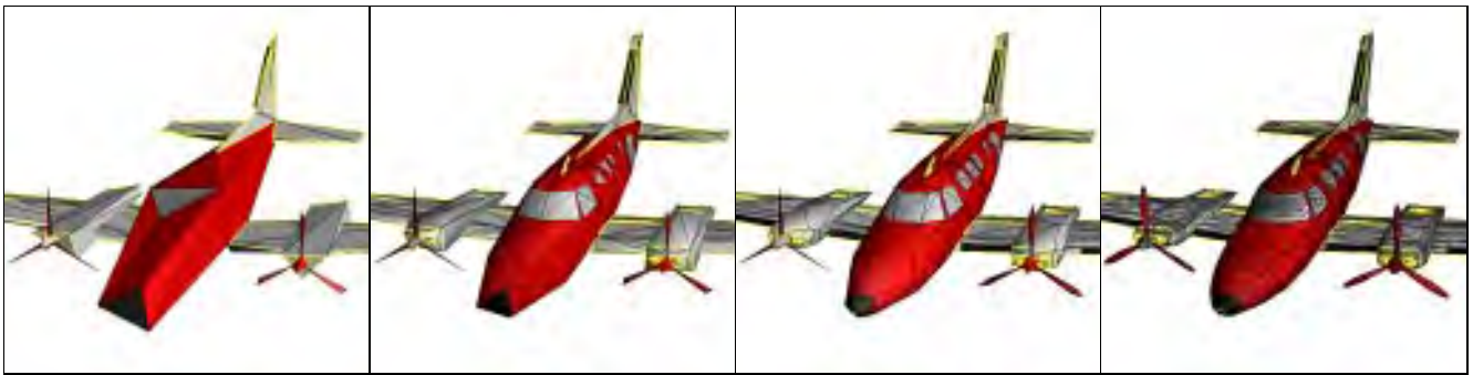
(a) Base mesh M^0 (150 faces) (b) Mesh M^{175} (500 faces) (c) Mesh M^{425} (1,000 faces) (d) Original \hat{M} = M^n (13,546 faces) Figure 5: The PM representation of an arbitrary mesh \hat{M} captures a continuous-resolution family of approximating meshes M^0 \dots M^n = \hat{M} .
