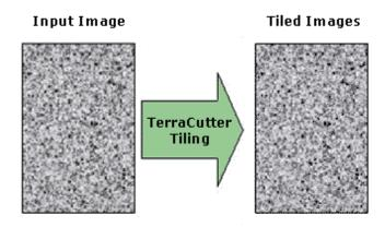
Conceptually, the process of loading data into TerraServer is simple. Tapes arrive from the USGS and SPIN-2 containing uncompressed image files. The files contain too much data to be downloaded over the Internet and are not in a format recognized by Web browsers, so they must be cut and merged with other images and compressed in the JPEG file format.
