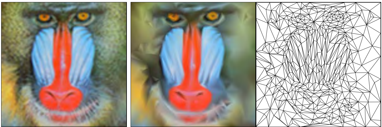
(a) M ( 200 \times 200 vertices) (b) Simplified mesh (400 vertices) Figure 8: Demonstration of minimizing E_{scalar} : simplification of a mesh with trivial geometry (a square) but complex scalar attribute field. ( \hat{M} is a mesh with regular connectivity whose vertex colors correspond to the pixels of an image.)
