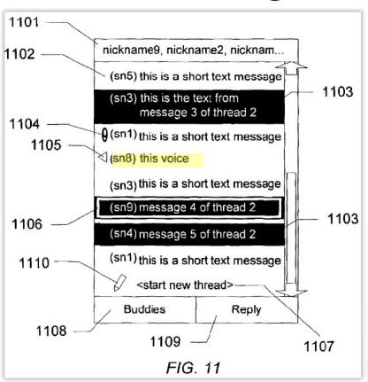
In the example of FIG. 11, each entry comprises an attachment indicator 1104-1105 that indicates if there is any attached content (e.g., documents, files, etc.) or transmitted speech available; the short name of the sender 705 or 803, and at least part of the message content or text (all of the text if the text fits within 2-3 lines). Although not illustrated in FIG. 11,
