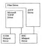
By binding the driver in this fashion, we can choose to direct incoming network data to our own ATCP transport driver, the Microsoft TCP driver, or both. We do this by playing with the ethernet "type" field as follows.
