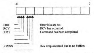
The setting of any bits in the ISR will cause an interrupt, provided the corresponding bit in the Interrupt Mask Register is set. The default setting for the IMR is 0.
