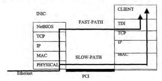
The transmit case works in much the same fashion. In slow-path mode the packets are given to the INIC with all of the headers attached. The INIC simply sends these packets out as if it were a dumb NIC. In fast-path mode, the host gives raw data to the INIC which it must carve into MSS sized segments, add headers to the data, perform checksums on the segment, and then send it out on the wire.
