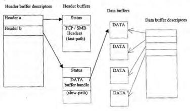
Since we want to fill in the header buffer with a single DMA, the header must be the last piece of data to be written to the host for any received transaction.
