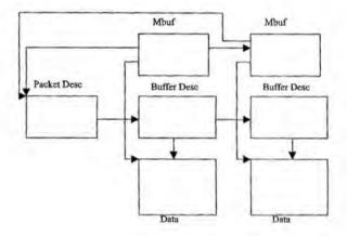
The mbuf structure will provide the standard fields provided in the FreeBSD mbuf including the data pointer, which points to the current location of the data, data length fields and flags. In addition each mbuf will point to the packet descriptor which is associated with the data being mapped. Once an NT packet is mapped, our transport driver should never have to refer to the packet or buffer descriptors for any information except when we are finished and are preparing to return the packet.
