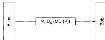
Fig. 7-24. Digital signatures using message digests.
