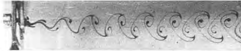
Figure 4.8 Vortex street in the wake of a cylinder (hidden by bracket) at Reynolds number of 5.5. (Reproduced with permission from Dr D J Tritton.)
