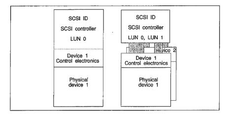
Figure 10.2 Embedded SCSI and bridge controllers.
