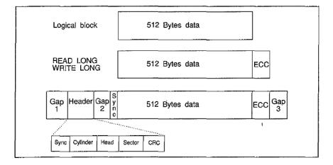
Figure 13.3 Physical layout of a logical block.
