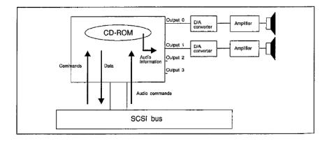
Figure 20.1 Model of a CD-ROM drive.
