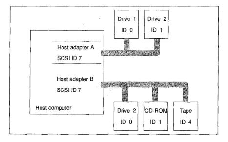
Figure 10.1 Computer with multiple SCSI buses.
