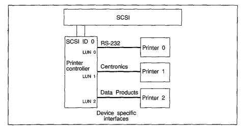
Figure 15.1 Model of a SCSI printer.
