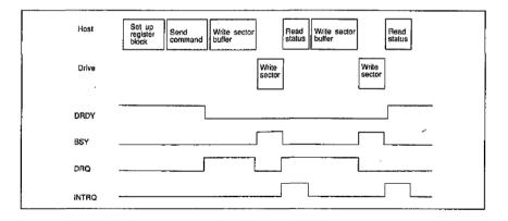
Figure 6.2 Timing of a class 2 command.
