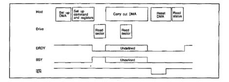
Figure 6.3 Timing of a class 4 command.
