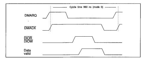
Figure 5.2 Timing diagram for single-word DMA.
