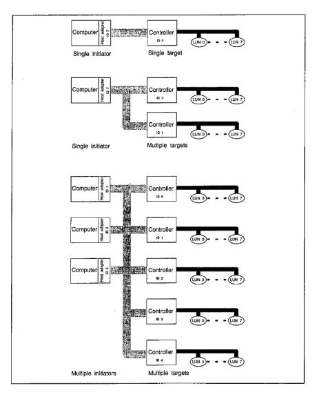
Figure 10.3 Basic SCSI configurations.
