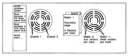
Figure 13.2 SCSI extends and notches.
