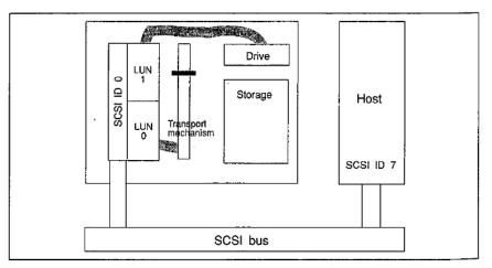
Figure 21.2 SCSI medium-changer configuration.
