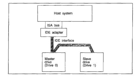
Figure 4.2 IDE configuration for AT compatibles.
