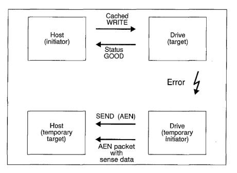
Figure 11.5 Asynchronous event notification.
