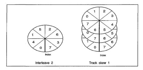
Figure 2.6 Interleave and track skew.
