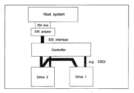
Figure 4.4 IDE configuration with bridge controller.
