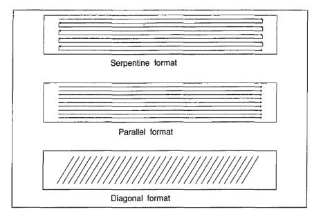
Figure 14.1 Various tape recording formats.
