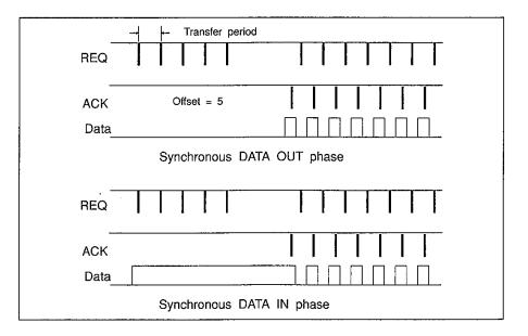
Figure 10.22 Synchronous data phases.
