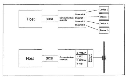
Figure 18.1 Examples of SCSI communications devices.
