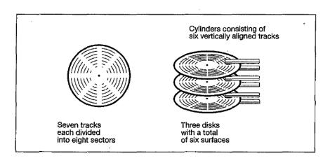
Figure 2.4 Structure of disk medium.
