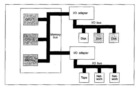
Figure 3.2 Computer system with multiple buses.
