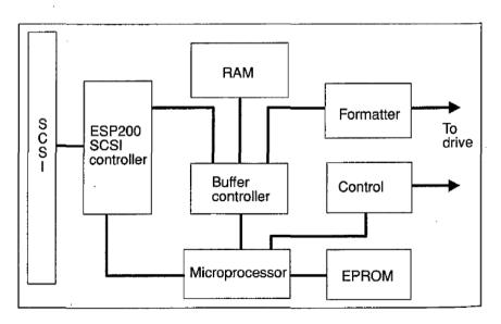
Figure 25.1 Typical target application using ESP200.
