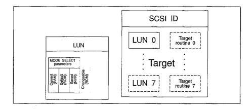
Figure 12.1 Model of a target.
