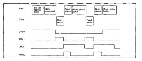
Figure 6.1 Timing of a class 1 command.
