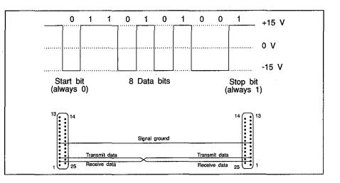
Figure 2.1 Physical interface: mini-RS-232.
