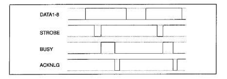
Figure 2.3 Centronics interface timing.
