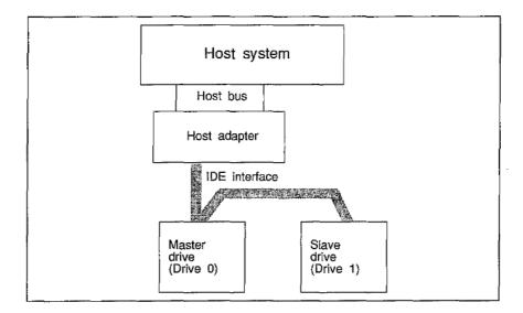
Figure 4.3 IDE configuration for AT compatibles.
