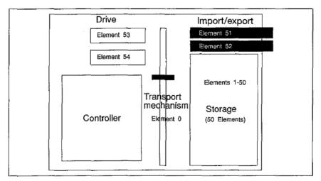
Figure 21.1 Model of a SCSI medium-changer device.
