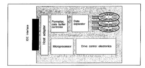
Figure 4.1 IDE drive block diagram.
