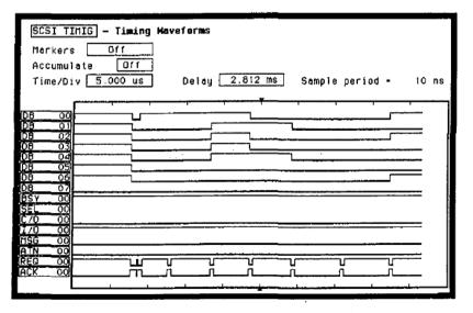
Figure 10.20 DATA phase as seen on a logic analyzer.
