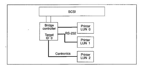
Figure 9.2 Bridge controller with logical units.
