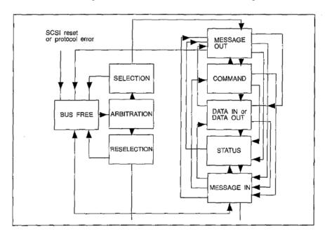
Figure 10.12 Complete SCSI phase diagram.
