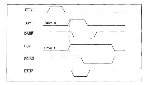
Figure 6.4 Timing at power-up or RESET.
