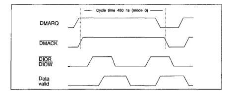
Figure 5.3 Timing diagram for multiple DMA transfers.
