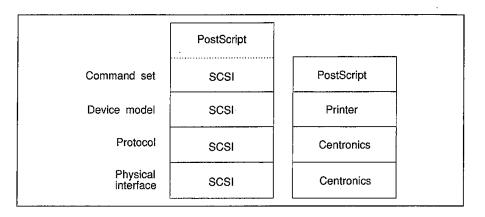
Figure 15.2 SCSI printer interface.
