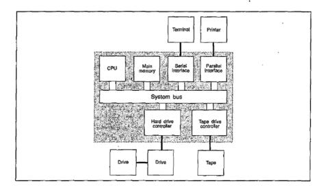
Figure 1.1 Computer system with peripheral devices.
