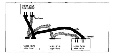
Figure 10.6 Mixed configuration with Wide SCSI.
