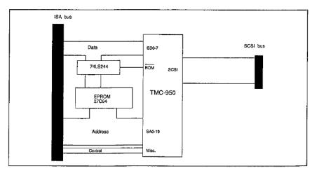
Figure 25.2 Three-chip PC host adaptor using TMC-950.
