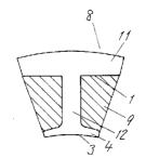
1 flat surface portion 3 rotor facing surface 4 pole shoe portion 8 unit core member 9 coil conductor 11 yoke portion 12 tooth portion
