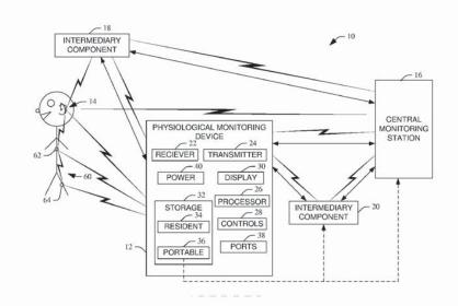
(57) Abstract: A portable physiological monitoring device (12) includes a receiver (22) that wirelessly receives physiological measurements from each of a plurality of in-the-ear probes (14) upon entering a communication range of one of the in-the-ear probes (14). The portable physiological monitoring device (12) farther includes a display (30) for presenting the physiological measurements.
