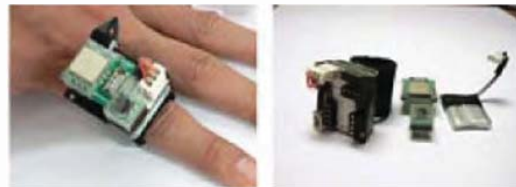
Fig. 1.Finger band sensor The wearable sensor device should be small and light
