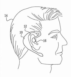
(57) Abstract: A physiological monitoring device (10) includes a device housing (11) shaped to fit behind an ear (12) of a subject and a sensor (18, 28, 30) attached to the device housing so as to sense a physiological characteristic of the subject at a location behind the ear. An earphone speaker (16) extends from the device housing towards an ear canal of the subject and provides an audible communication to the subject responsively to the physiological characteristic.
