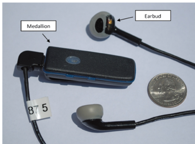
FIGURE 1 The components and size of the device under test (DUT). Shown are the earbud and the medallion containing the majority of the computational components. Shown for scale is a U.S. quarter. Note the position of the sensor module at the bottom of the antitragus. The sensor module is configured to fit between the concha and the antitragus of the ear.
