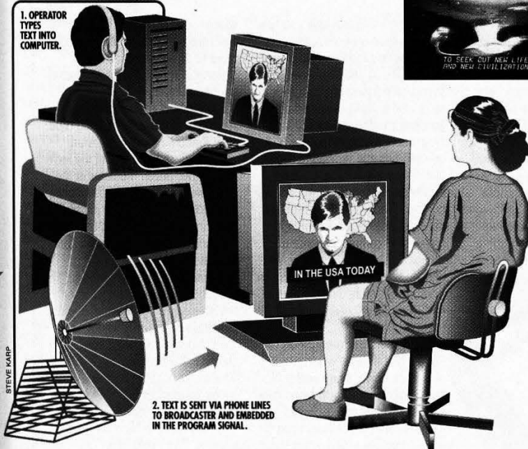
3. TV SET DECODES CAPTION AND DISPLAYS TEXT AT BOTTOM OF SCREEN.
