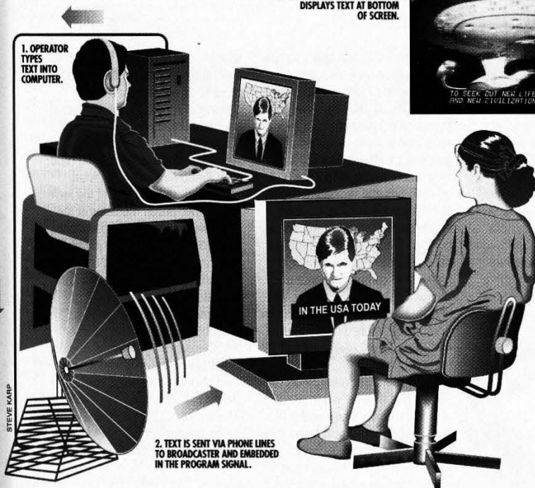
Text is input and broadcast in synchronization with the audio portion of a prerecorded show or within seconds of a live broadcast. A caption-ready TV set is needed to display the text.
