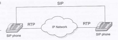
specifically to ensure transport (RTP), provide signaling with the PSTN, guarantee voice quality (Resource Reservation Setup Protocol [RSVP]), provide directories (Lightweight Directory Access Protocol [LDAP]), authenticate users (Remote Access Dial-In User Service [RADIUS]), and scale to meet anticipated growth curves.
