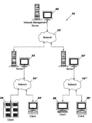
Figure 1 illustrates a computer network according to an embodiment of the invention. *Id.* at 6:60–63. In particular, network management server 20 is connected to on-demand servers 22 and 22' which are in turn connected to client stations 24 and 24' and 26 and 26' respectively. *Id.* at 6:63–7:9. The '293 patent describes a method of distributing software from the network management server to the on-demand servers. *Id.* at 17:20–18:36.
