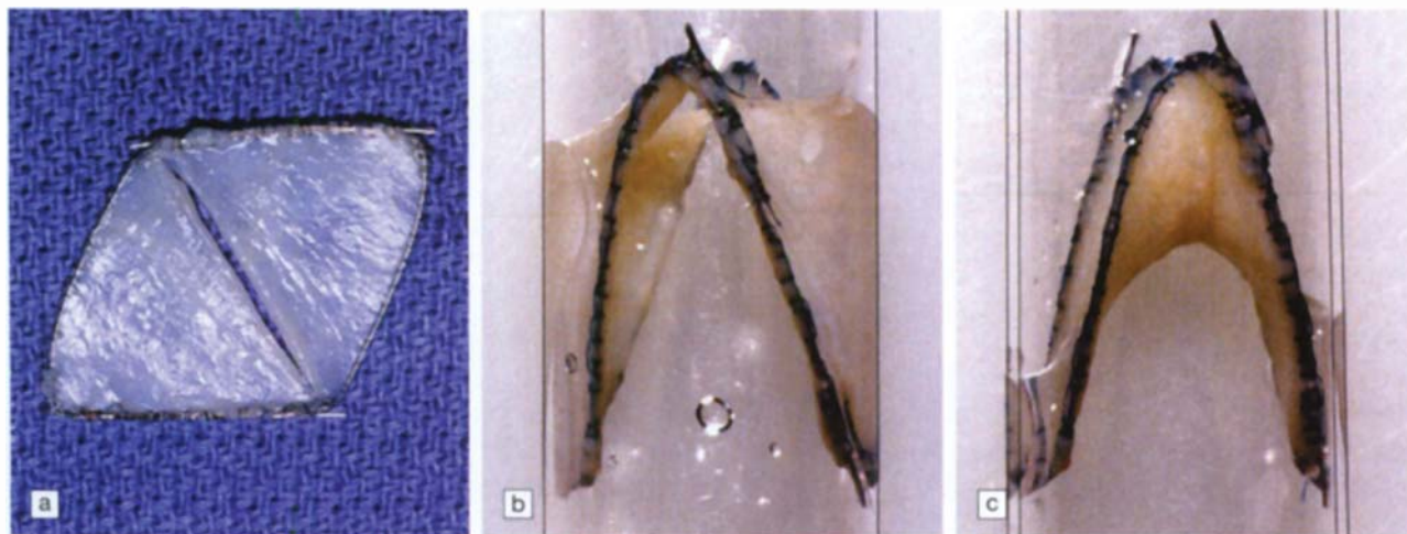
Figure 2. Valve design. (a) Non-restricted valve 20 mm in length with four barbs. (b) Deployed valve in a plastic tube, open position. (c) Deployed valve in a plastic tube, closed position.
