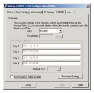
WEP (Wired Equivalent Privacy) is a data privacy mechanism based on a 40 bit shared key algorithm, as described in the IEEE 802.11b standard. In order to utilize WEP encryption, all points in your wireless network must have WEP enabled and be set to the same Key Setting. For easier configuration, it is strongly recommended that you use the Passphrase feature.
