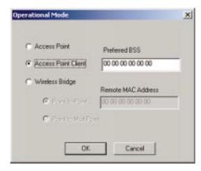
Wireless Bridge - If you are trying to make a wireless connection between two or more wired networks, select Wireless Bridge. There are two options: Point to Point and Point to MultiPoint.
