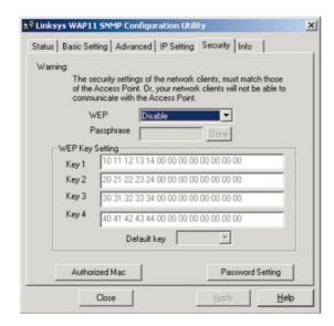
WEP (Wired Equivalent Privacy) is a data privacy mechanism based on a 64/128-bit shared key algorithm, as described in the IEEE 802.11 standard. In order to utilize WEP encryption, all points in your wireless network must have WEP enabled and be set to the same Key Setting.
