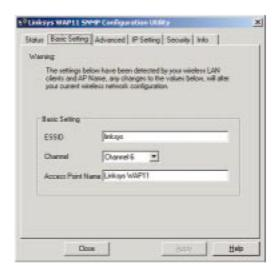
The Wireless Network Access Point will automatically detect the settings to your wireless network. Changing these values will alter your current wireless network configuration.
