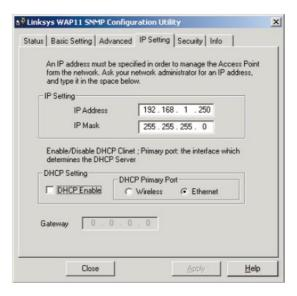
The IP settings for the Access Point are made from this tab. This is for the SNMP Configuration Utility use only.
