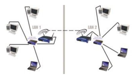
To configure a Point to Point bridged environment:
