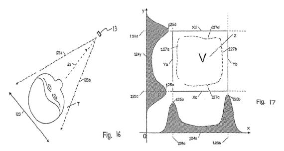
Figure 16, above, depicts camera 13 viewing a head. Ex. 1001, 22:19–23. Figure 17 depicts x axis and y axis histograms of a head from a video conference. *Id.* at 8:66–67, 22:4–6, 22:55–67. Face V is approximately defined by the peaks in the two respective histograms. *Id.* at 23:1–9. Figure 22 of the '134 patent is reproduced below.
