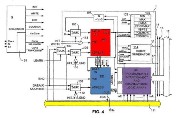
According to the '293 patent, in the self-adapting embodiment illustrated in Figure 4, the content of the memory of classifier 101 is updated automatically. Ex. 1001, 11:14–29. To implement the self-adapting function (i.e., real-time updating of classifier 101), classifier 101 has an
