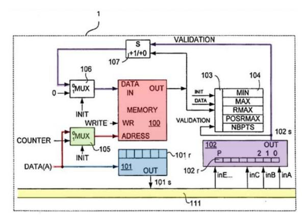
As shown in highlighted Figure 3 above, histogram calculation unit 1 includes analysis memory 100 (highlighted in red), address multiplexer 105 (highlighted in green), data input multiplexer 106, incrementation unit 107, classifier 101 (highlighted in blue), time coincidences unit 102 (highlighted in purple), and test unit 103, which is connected to analysis output registers 104. Ex. 1001, 8:37–43, 9:51–54. Output of classifier 101 is connected to bus 111 (highlighted in yellow). *Id.* at 9:36.
