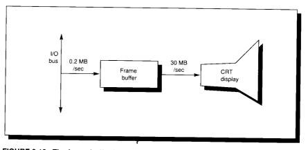
FIGURE 9.18 The frame buffer is connected to both the I/O bus and the display. Because of the high data rate from the buffer to the display, the frame buffer is frequently dual ported.
