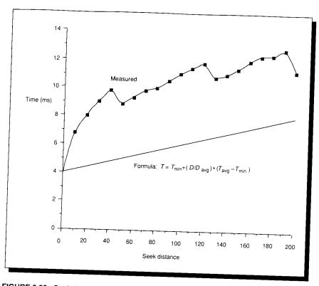
**FIGURE 9.38** Seek time versus seek distance for the first 200 cylinders. The Imprimis Sabre 97209 contains 1.2 GB using 1635 cylinders and has the IPI-2 interface [Imprimis 1989]. This is an 8-inch disk. Note that longer seeks can take less time than shorter seeks. For example, a 40-cylinder seek takes almost 10 ms, while a 50-cylinder seek takes less than 9 ms.
