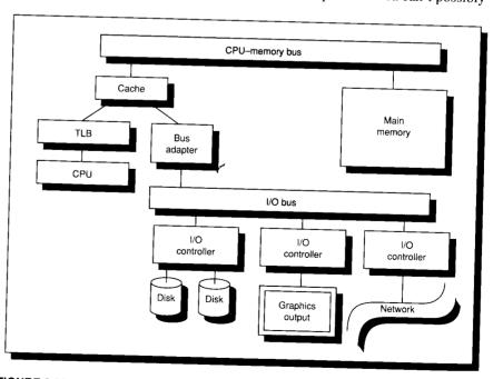
FIGURE 9.28 Example of I/O connected directly to the cache.
