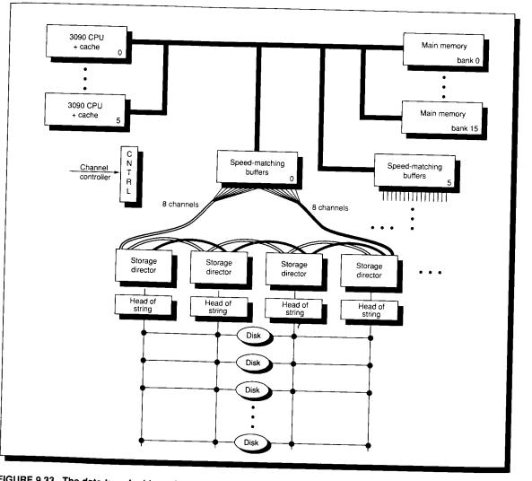
**FIGURE 9.33** The data-transfer hierarchy in the IBM 3990 I/O Subsystem. Note that all the channels are connected to all the storage directors. The disks at the bottom represent the quad-ported IBM 3380 disk drives, with the maximum of 64 disks. The collection of disks on the same path to the head-of-string controller is called a *string*.
