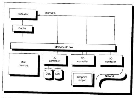
FIGURE 9.1 Typical collection of I/O devices on a computer.
