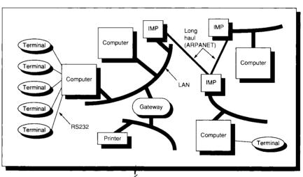
FIGURE 9.23 A computer system today participates in a hierarchy of networks. Ideally, the user is not aware of what network is being used in performing tasks. The gateway routes packets to a particular network, a network routes packets to a particular host computer, and the host computer routes packets to a particular process.
