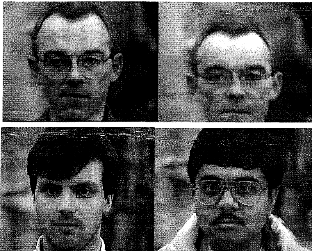
Figure 4. Snapshots from the system during tracking. Note that in the second image, the system missed tracking of one eye.
