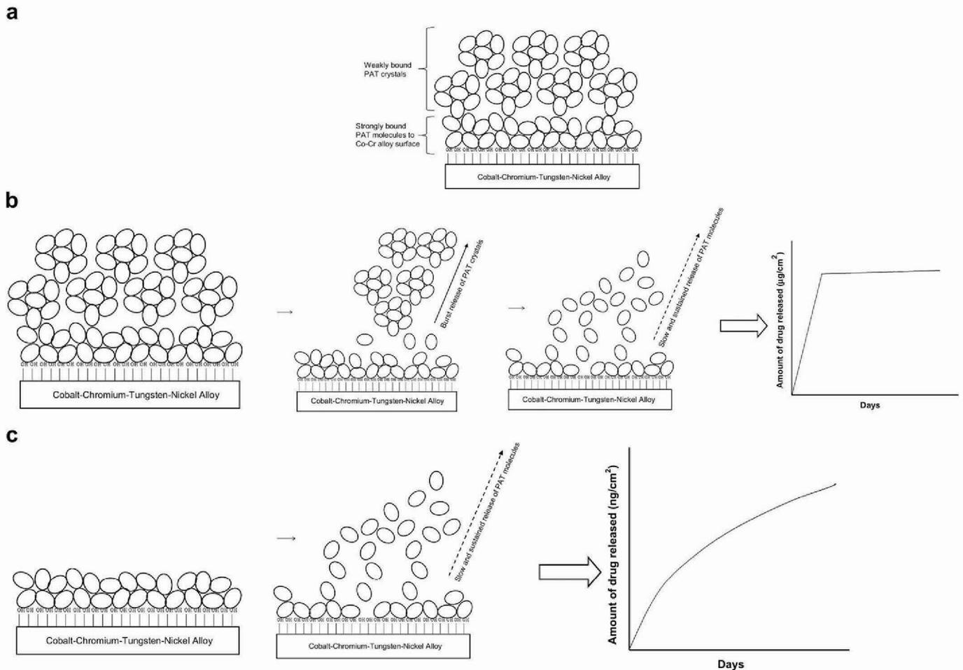
**Fig. 10.** (a) Schematic of the formation of PAT coating on Co–Cr alloy, (b) Schematic of the drug release from Groups C and D – Initial burst release of PAT crystals followed by a slow and sustained release of PAT molecules, (c) Schematic of the drug release from Groups A and B – Slow and sustained release of PAT molecules.
