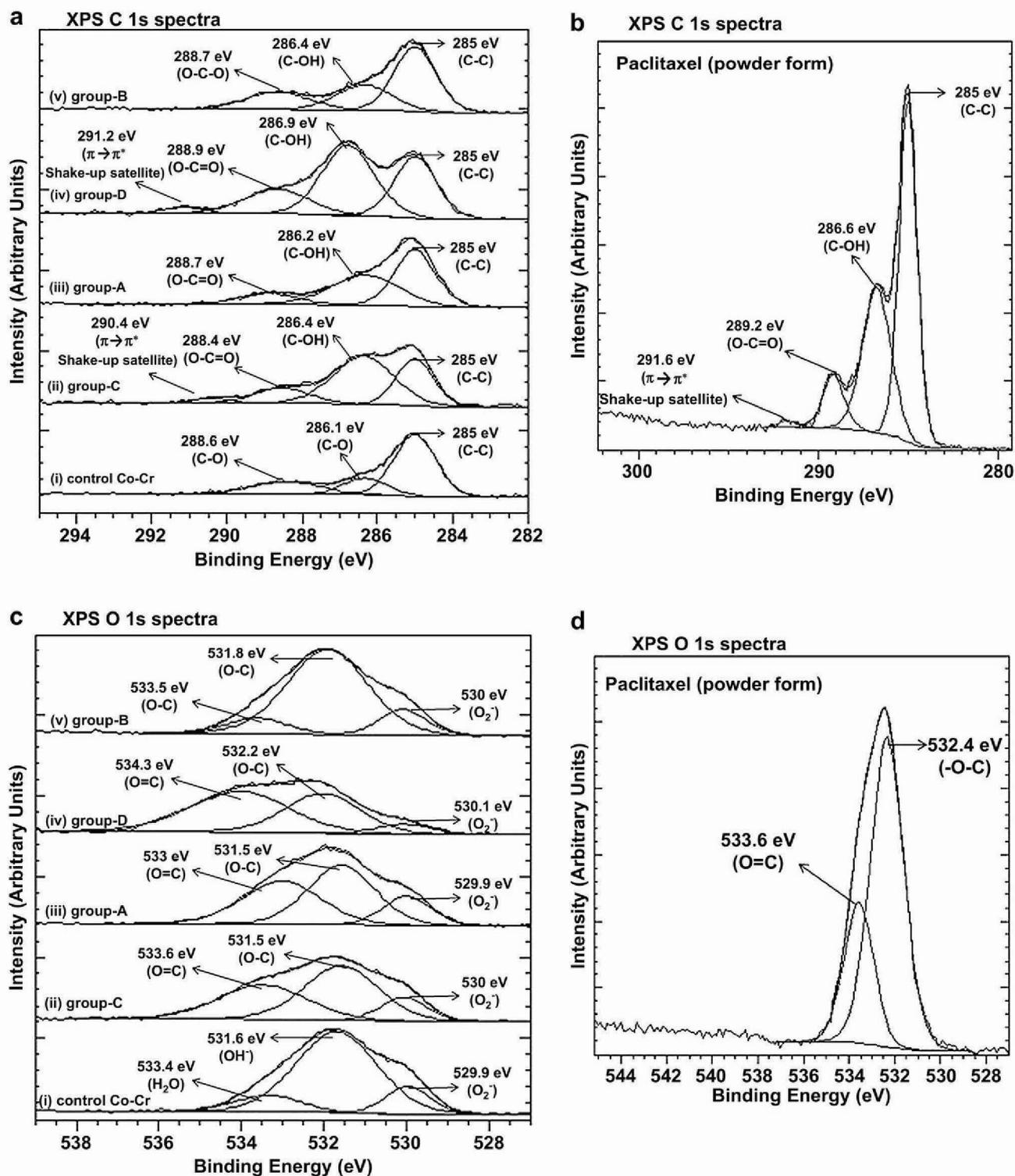
**Fig. 9.** XPS C 1s spectra of control Co–Cr and groups-A to D (a); C 1s spectrum of paclitaxel (powder form) (b); O 1s spectra of control Co–Cr alloy and groups-A to D (c); and O 1s spectra of paclitaxel (powder form) (d).
