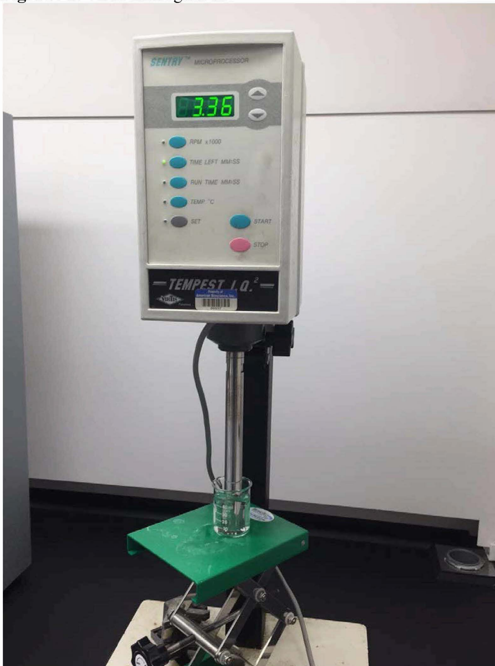
Figure 2a. Virtis homogenizer
