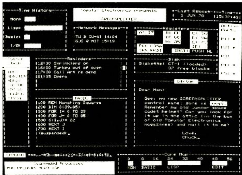
The Screensplitter can generate almost any number of independent "windows" contingent on the needs of the user.
