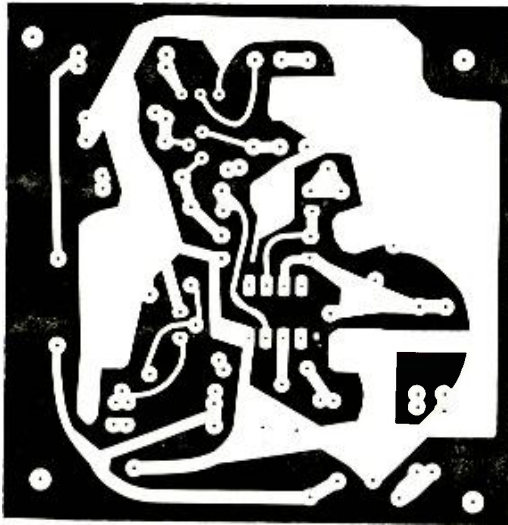
Fig. 3. Actual-size etching and drilling guide is shown at left. Component placement guide is above.
