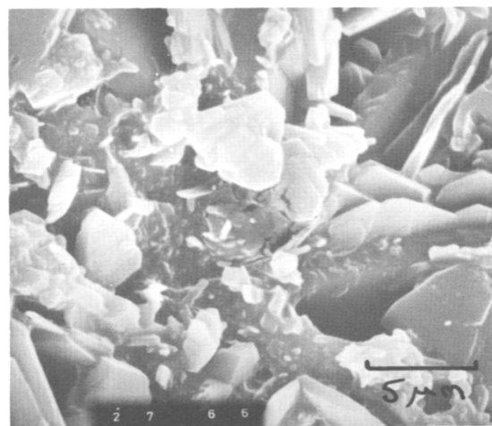
Fig. 3. Scanning electron micrographs of a Celutab particle (710 - 1000- \mu\text{m} sieve fraction).
