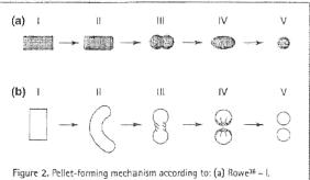
rigure 2. reliet-forming mechanism according to: (a) Nowe's - I. Cylinder; III. Cylinder with rounded edges; III. Dumb-bell; IV. Ellipse; V. Sphere. (b) Baert - I. Cylinder; II. Rope; III. Dumb-bell; IV. Sphere with a cavity outside; V. Sphere. [Reproduced with permission from Ref. 9.]
