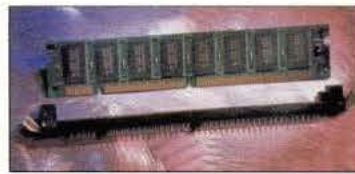
SDRAM MODULES such as this Hitachi part ease upgrade problems by meeting industry standards.
