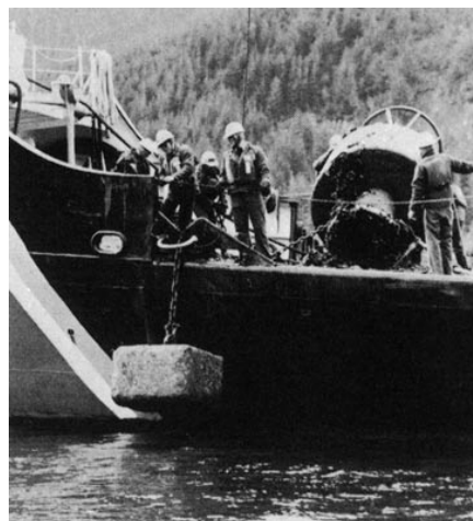
Figure 512. A sinker used to anchor a buoy.
