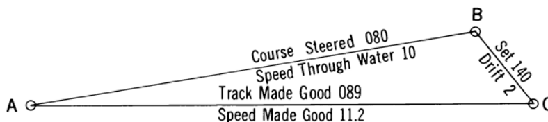
Figure 708a. Finding track and speed made good through a current.
