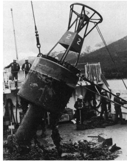
Figure 509. Buoy showing counterweight.
