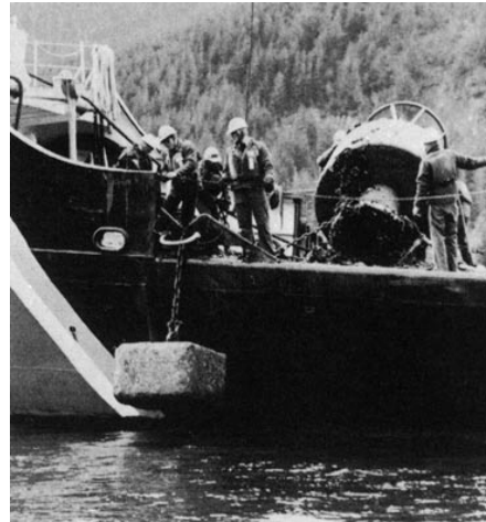
Figure 512. A sinker used to anchor a buoy.
