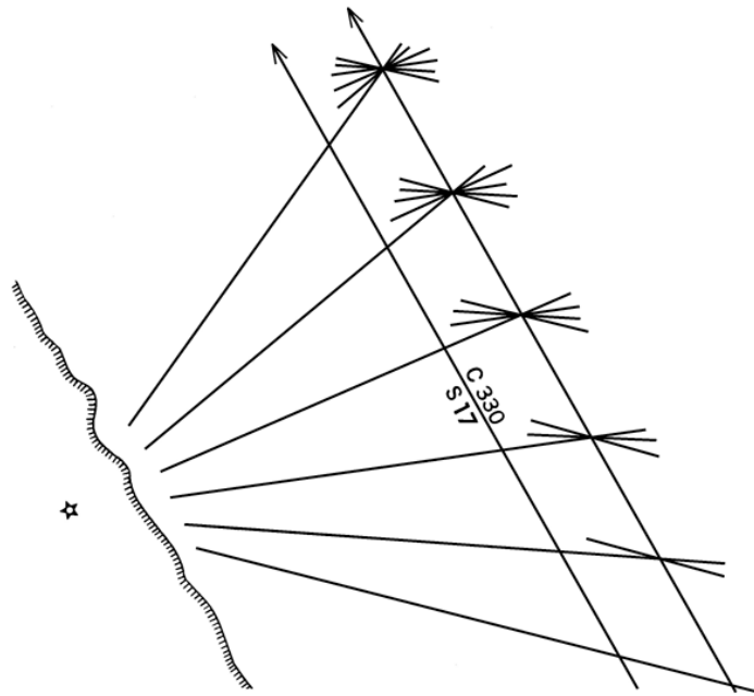
Figure 819b. A number of running fixes with a following current.
