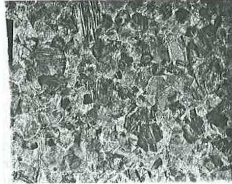
Fig. 1.2 Micrograph of polycrystalline silicon. The crystallites are called grains and the regions between the grains are called grain boundaries. (Courtesy: W. Tice, IBM).
