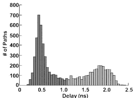
Fig. 3. Histogram of path delays with Al interconnects.
