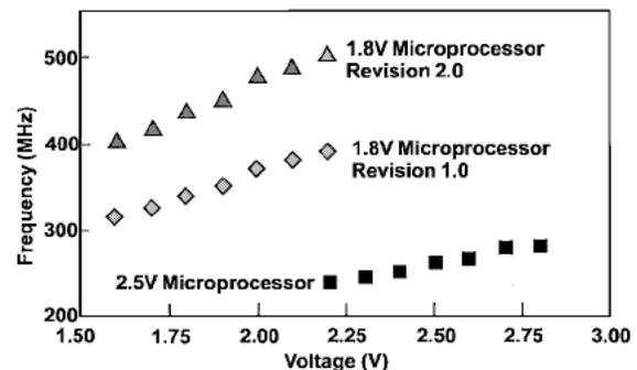
Fig. 10.  $F_{max}$  versus voltage for critical path delays.
