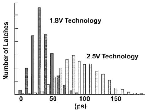
Fig. 6. Clock skew of all falling C1.
