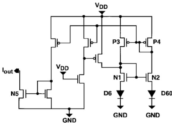
Fig. 7. Voltage reference circuit.
