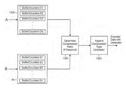
As shown above in Figure 13B of the '513 patent, "compression ratio module 1340, operatively connected to the content dependent output
