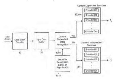
As shown above in Figure 13A of the '513 patent, the system receives an input data stream of data blocks. *Id.* at 15:63–16:5. Content dependent data recognition module 1300 analyzes the incoming data stream to recognize
