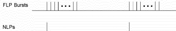
Figure 28-3—FLP Burst sequence to NLP sequence mapping
