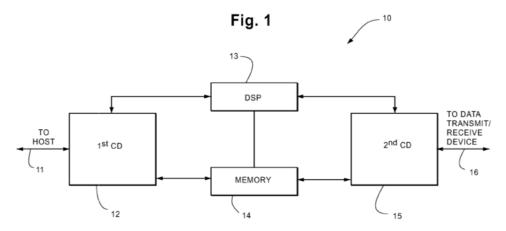
As shown in Figure 1, interface device 10 connects to a host device via host line 11, and to a data transmit/receive device via output line 16. *Id.* at 5:47–63. Interface device 10 includes first connecting device 12, second connecting device 15, digital signal processor 13, and memory means 14.
