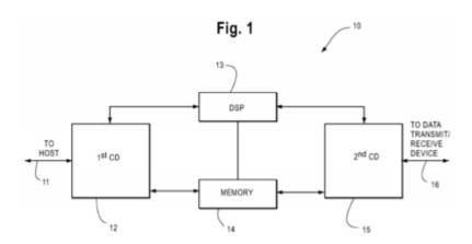
As shown in Figure 1, interface device 10 connects to a host device via host line 11, and to a data transmit/receive device via output line 16. *Id.* at 4:62–5:10. Interface device 10 includes first connecting device 12,
