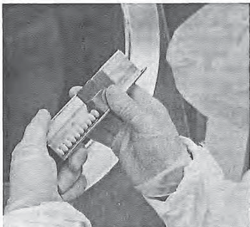
Fig. 5-52. Tablet gauge used to measure the size of coated tablets. (Courtesy of Eli Lilly and Company.)
