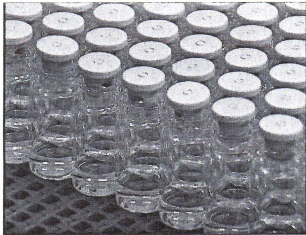
Figure 10-1 Partially slotted stoppers in solution vials prior to loading into freeze-dryer.
