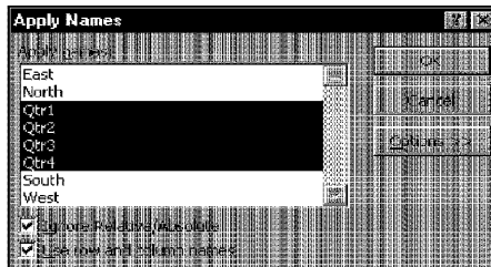
Figure 9-19: The Apply Names dialog box lets you replace cell or range references with names.
