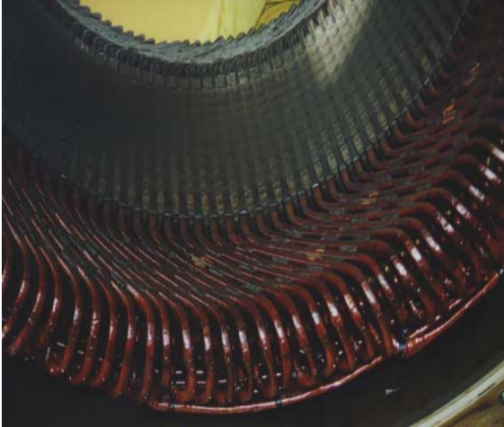
COILS WOUND IN STATOR FOR A REACTOR COOLANT PUMP MOTOR
