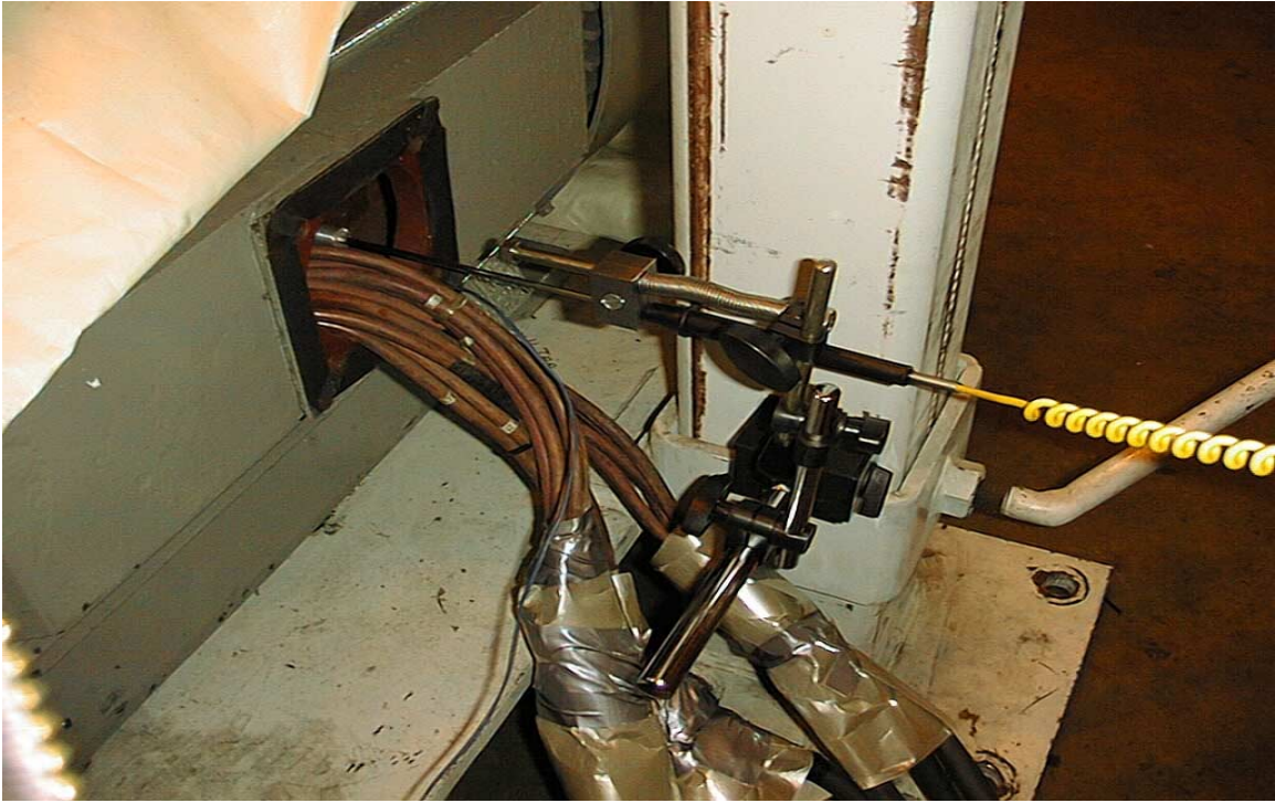
SPECIAL MAGNETIC BASE AND SPRING LOADED THERMOCOUPLE BEING USED ON MOTOR BACK IRON - THIS MOTOR DID NOT HAVE EMBEDDED TEMPERATURE ELEMENTS
