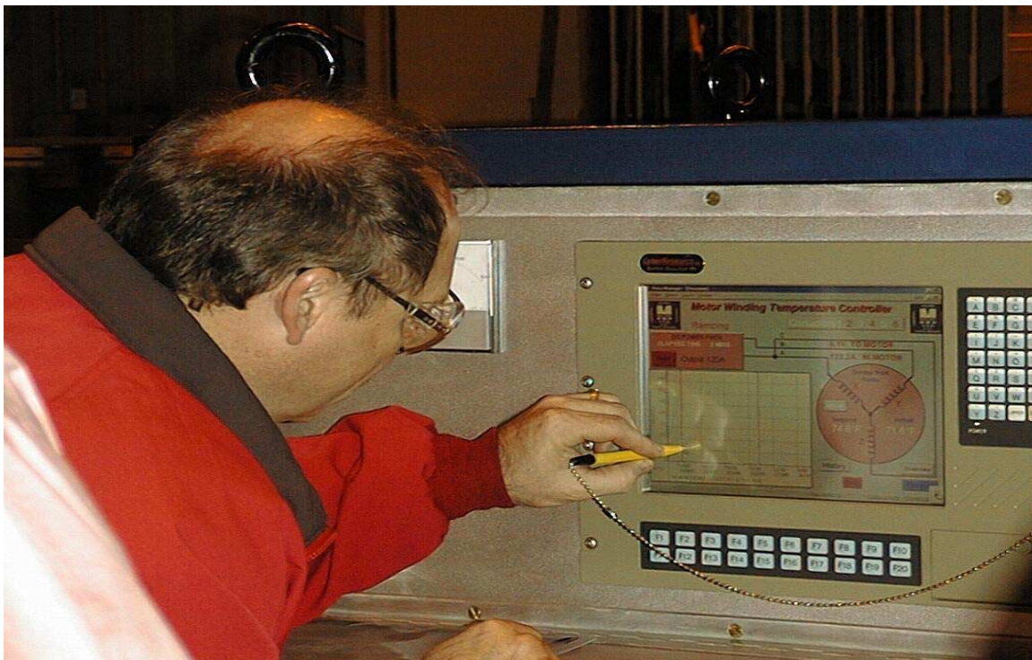
DISPLAY OF ADM DURING OPERATION NOTICE TOUCH SENSITIVE SCREEN
