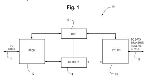
As shown in Figure 1, interface device 10 connects to a host device via host line 11, and to a data transmit/receive device via output line 16. *Id*.
