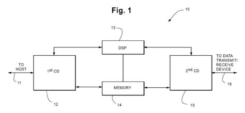
As shown in Figure 1 above, interface device 10 connects to a host device via host line 11, and to a data transmit/receive device via output line 16. *Id.* at 5:47–63. Interface device 10 includes first connecting device 12, second connecting device 15, digital signal processor 13, and
