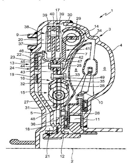
The figure above "shows a hydrodynamic torque converter disposed about a rotation axis in a half-sectional view." *Id.* at 3:52–55. Torque converter 1 includes torsional vibration absorber 17, torsional vibration damper 16, damper stage 14, and damper stage 15. *Id.* at 4:37–38; 5:3–5.
